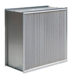
Filtro HEPA Standard Capacity (SC) & High Capacity (HC) filters are pleated aluminium separator filters with efficiencies ranging from H12 to H14 grades. These filters generally come in wood and metal constructions. Box type or double turned flanged version available.
